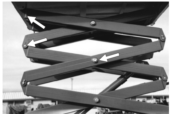
Figure 7.19 - Structural Damage and Welds
