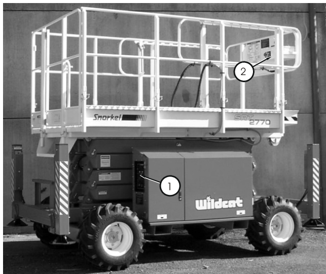
Figure 6.1 - Control Box Locations
