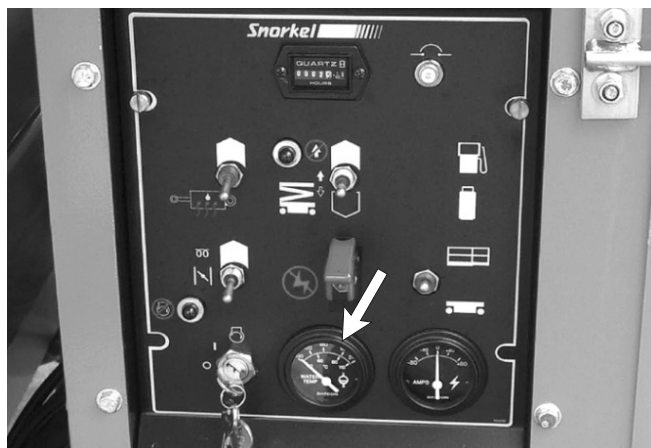
Figure 4.1 - Water Temperature Gauge
